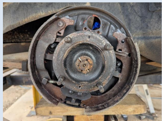
Ed. Front brakes, above, getting back together, rear brakes, right, coming apart.
