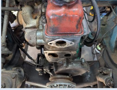
Ed. Alternator, water pump, thermostat housing removed.
