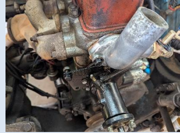
Ed. Water pump and thermostat housing in place – I had mastered the torque wrench by this stage!
